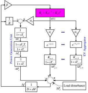
Fig. 2. General model of modified LFC system
