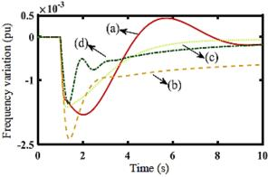
Fig. 14. Frequency variation of the LFC scheme(a) PSO-PID (b) SCA-PID (c) PSO-FOPID (d) SCA-FOPID for  $\tau(t) = e^{-2.3t}$
