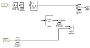
Fig. 17. The proposed switching logic for ESS
