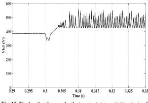
Fig. 15. The bus 3 voltage under the transient state switching logic of ESS (case 5)
