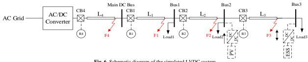
Fig. 6. Schematic diagram of the simulated LVDC system
