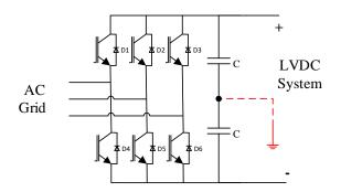
Fig. 7. Model of the controlled rectifier
