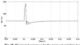
Fig. 18. PV injected current under the proposed switching logic (Ipv=70 A)
