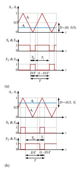
Fig. 2. The control signals, (a) in D = [0, 0.5) operating zone, (b) in D = (0.5, 1] operating zone.
