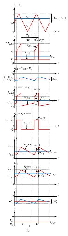
Fig. 5. Waveforms of the proposed converter, (a) operating zone of D = [0, 0.5), (b) operating zone of D = (0.5, 1].
