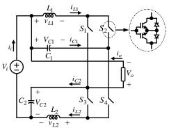
Fig. 1. The proposed buck-boost Z-source converter.
