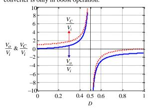
Fig. 4. Variations of the voltage gain and stress voltage on capacitors in terms of duty cycle.
