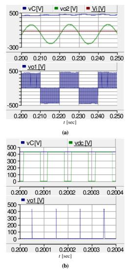
**Fig. 12.**Steady state performance of the proposed inverter, (**a**) input voltage  $(V_i)$ , capacitor voltage  $(V_C)$ , load voltage  $(V_{o2})$  and the output voltage of inverter  $(V_{o1})$ , (**b**) capacitor voltage  $(V_C)$ , input voltage of the inverter  $(V_{dc})$  and the output voltage of the inverter  $(V_{dc})$
