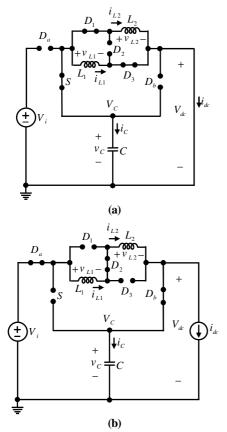
Fig. 2.The equivalent circuits of the proposed topology in different operating modes, (a) in the time interval of  $D_{ST}$ T<sub>s</sub>, (b) in the time interval of (1-  $D_{ST}$ )T<sub>s</sub>
