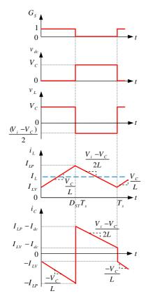
Fig. 3.The steady state waveforms of proposed Z-source inverter in CCM
