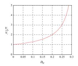
Fig. 4. Variation curve of  $V_C / V_i$  versus  $D_{ST}$  in the proposed Z-source inverter
