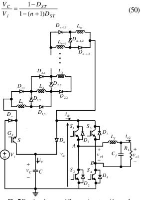
**Fig. 7.**Developed proposed Z-source inverter with n - 1 switched cells
