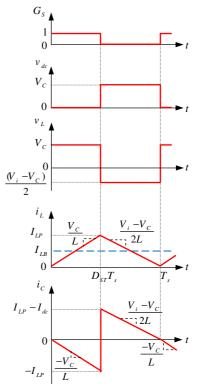
Fig. 5.Steady state waveforms of the proposed inverter in boundary operating
