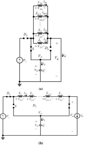
Fig. 8. The equivalent circuits of the developed inverter in different operating modes, (a) in the time interval of  $D_{ST}$ T<sub>s</sub>, (b) in the time interval of (1-  $D_{ST}$ )T<sub>s</sub>
