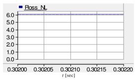
Fig. 14.The power losses of switches and diodes in nonload condition (Switching losses)
