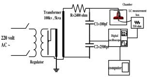
Fig. 1. A schematic of the experimental setup.
