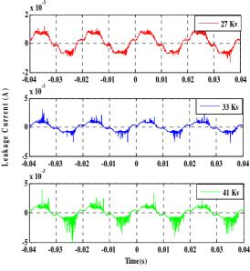
Fig. 7. Leakage current waveforms of insulator 1 in various voltage levels (27, 33 and 41 kV), humidity=77%, medium pollution levels.
