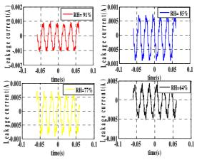
Fig. 6. Leakage current waveforms versus different levels of humidity (RH %) for insulator number 3.
