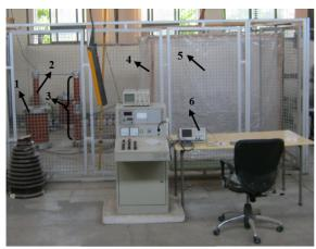
Fig. 4. Image of experimental setups. 1. HV transformer, 2. HV resistance, 3. Capacitive divider, 4. Fog chamber, 5. Insulator sample, 6. Oscilloscope.
