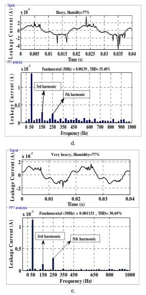
Fig. 5. Waveforms of the leakage current and FFT of insulator number 1 in various pollutions at 77% humidity.
