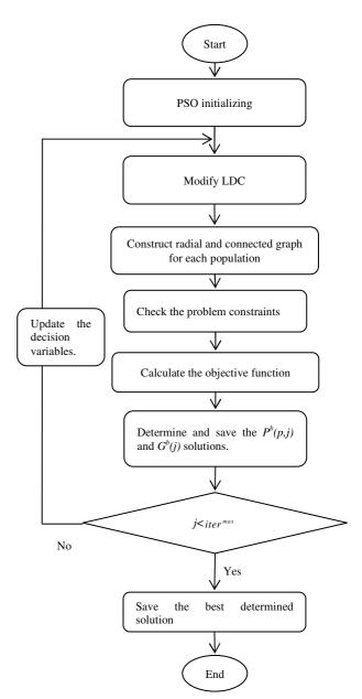
Fig. 3. Overall scheme of the optimization process
