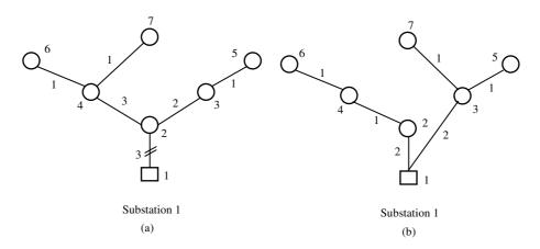
Fig. 5. 7-node test system design: a) in the absence of DRRs b) in the presence of DRRs
