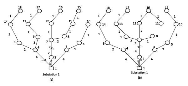
Fig. 8. 18-node test system design: a) in the absence of DRRs b) in the presence of DRRs
