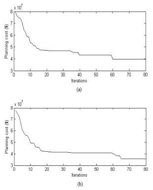
Fig. 9. PSO Optimization stages for 18-node test system: a) DEP problem, b) SDEP problem
