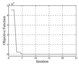
Fig. 6. Convergence curve of FWSOA method for IEEE 14-bus system
