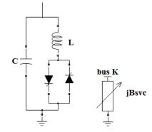
Fig. 1. General circuit structure for SVC [11]
