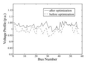
Fig. 7. Voltage profile for IEEE 57- bus test system before and after optimization.
