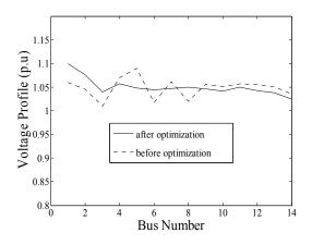
Fig. 5. Voltage profile for IEEE 14- bus test system before and after optimization.
