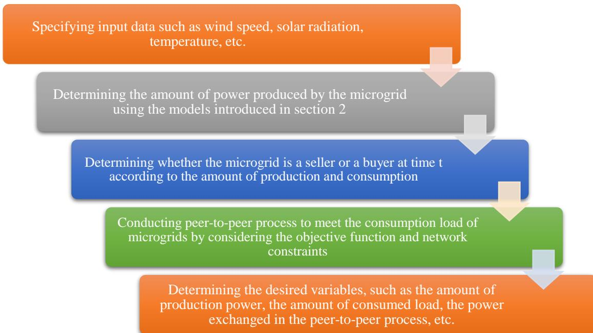
Fig. 3. Solution methodology flowchart
