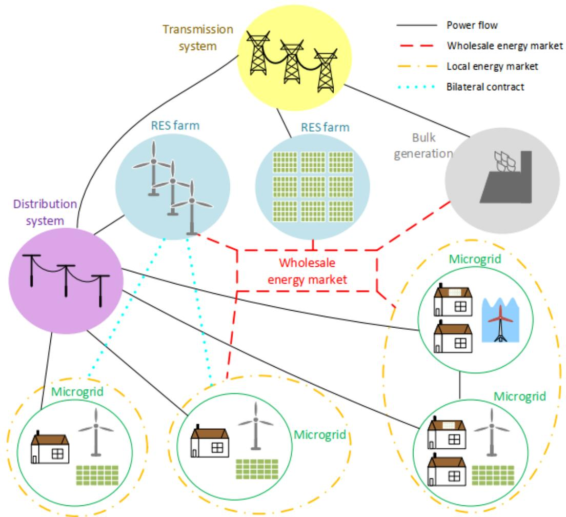
Fig. 2. Trading power between different members in a power network [2]
