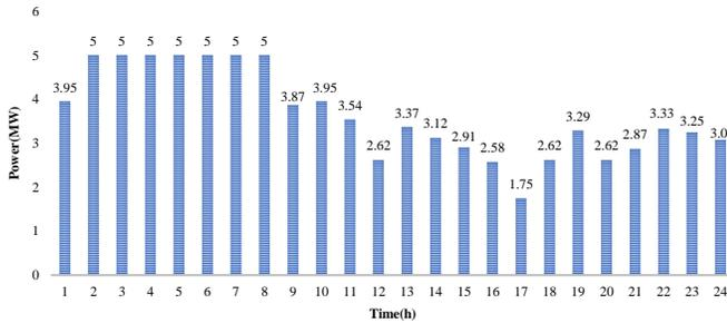
Fig. 7. Power generated by wind turbine
