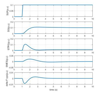
Fig. 9. Damping process of frequency oscillations of the studied system in Scenario 2
