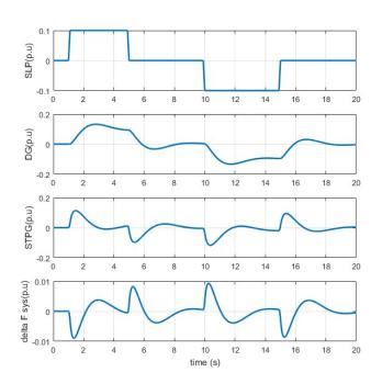
Fig. 8. Damping process of frequency oscillations of the studied system in Scenario 1 for variable load
