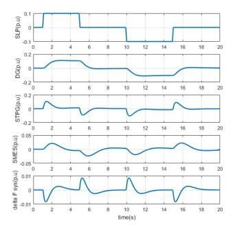
Fig. 10. Damping process of frequency oscillations of the studied system in Scenario 2 for variable load
