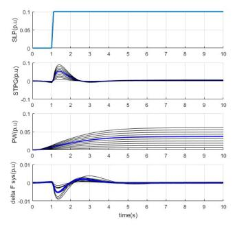
Fig. 13. Damping process of frequency oscillations of the studied system in Scenario 4
