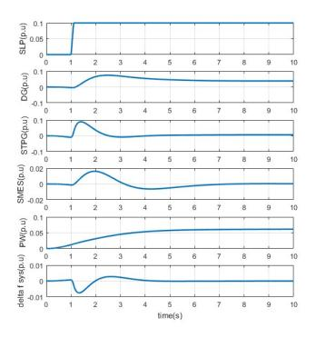
Fig. 11. Damping process of frequency oscillations of the studied system in Scenario 3
