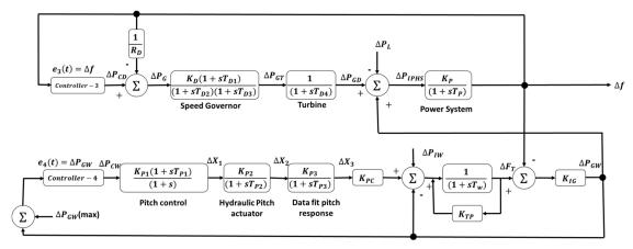
Fig. 2. Block diagram of the grid-connected hybrid power system.
