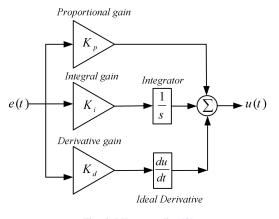
Fig. 5. PID controller [8]
