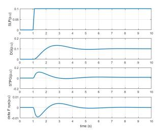
Fig. 7. Damping process of frequency oscillations of the studied system in Scenario 1
