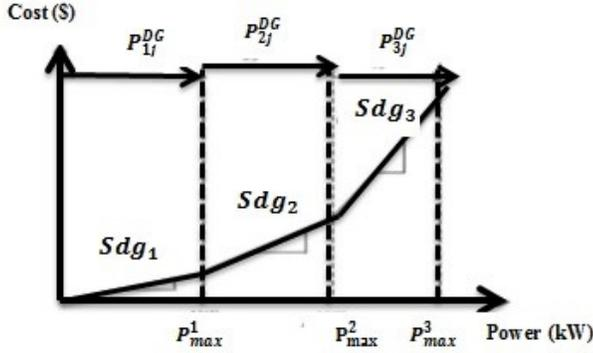
Fig. 3. Linear operation cost model of DG units [33].
