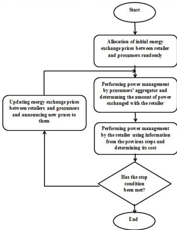
Fig. 4. The flowchart of the proposed algorithm
