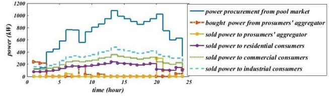
Fig. 9. The power procurement of the retailer in FP method (case 2a)
