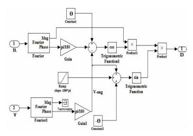
Fig. 3. Block diagram for generating  $I_D$ .
