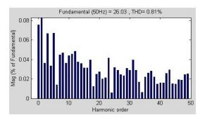
Fig. 8. Harmonic spectrum of grid current phase 'a' for SPEA2 technique.
