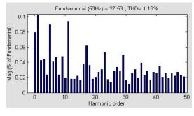
Fig. 7. Harmonic spectrum of grid current phase 'a' for NSGA-II technique.
