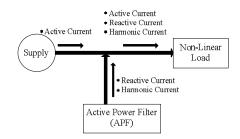
Fig. 1. Connection of shunt active filter with nonlinear load
