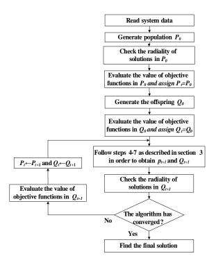
Fig. 1. The flowchart of the proposed NSGA-II
