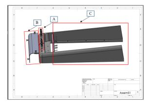
Figure 2: Technical Map of the swimming start block reaction time device
