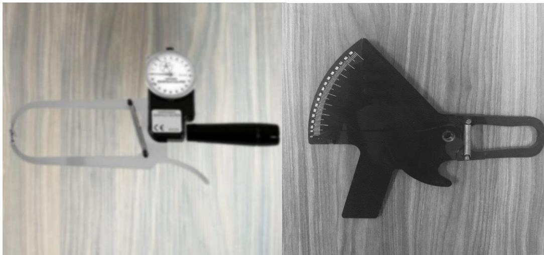
**Fig. 2.** Iranian slim guide caliper vs Harpenden caliper
