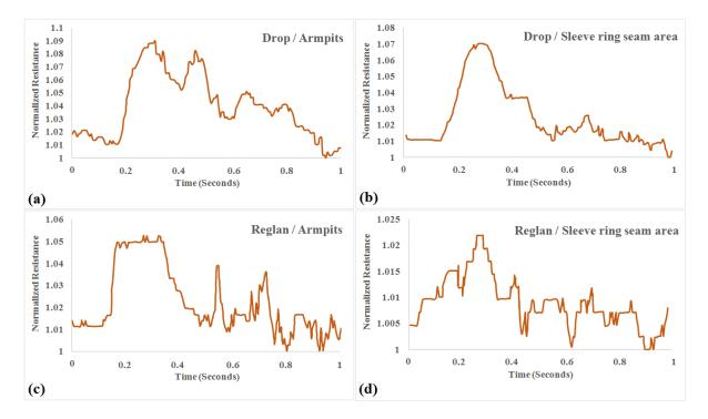
**Figure 10.** Metal yarn resistance variations for (a) drop sleeves with the metal yarn on the armpits, (b) drop sleeves with the metal yarn near the seam, (c) raglan sleeves with the metal yarn on the armpits, and (d) raglan sleeves with the metal yarn near the seam (normalized resistance is the division of resistance at any time to the resistance of the non-extended state)
