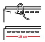
Figure 5. Schematic of the sewing condition of the metal yarn.
