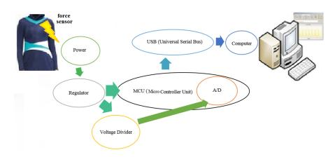
Figure 7. Electronic circuit components recording the tension variations.
