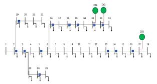
Fig. 6. Optimal location of automatic switches and DGs in the network obtained in CORP for  $\beta = 0.001$
