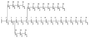
Fig. 3. IEEE 33 bus network schematic
