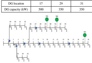
Fig. 5. Optimal location of automatic switches and DGs in the network obtained in SORP
