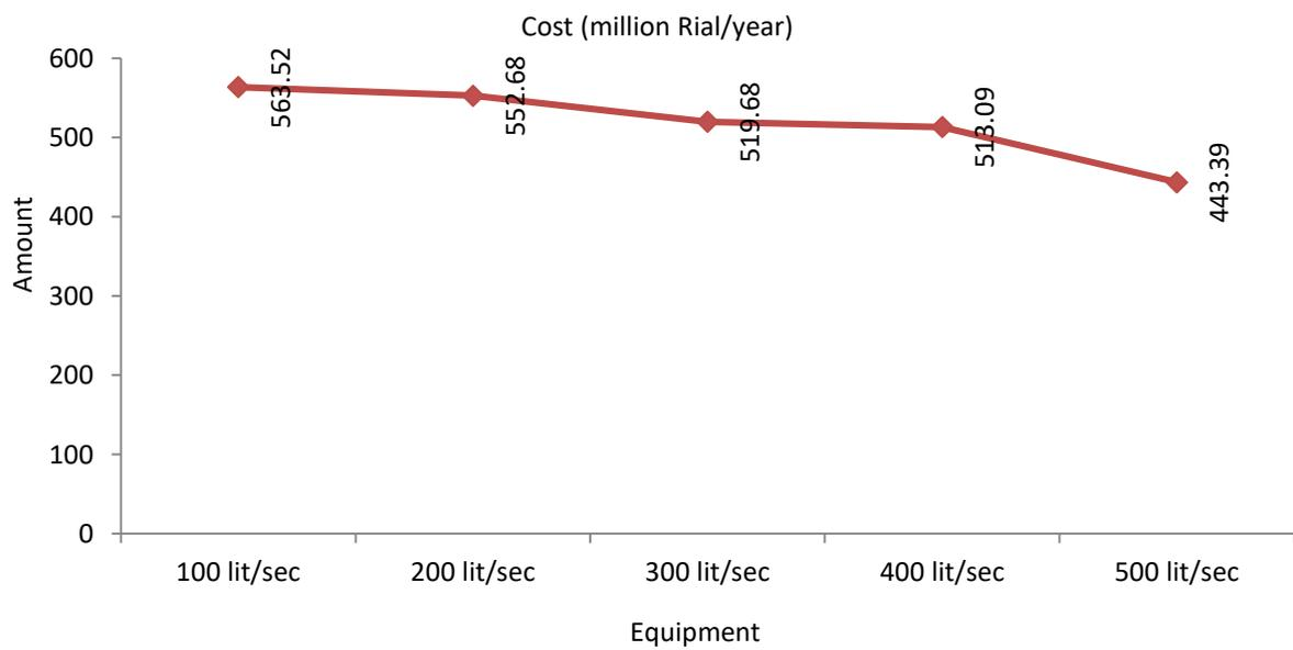
Fig. 12. Comparison of design costs for different water flows
