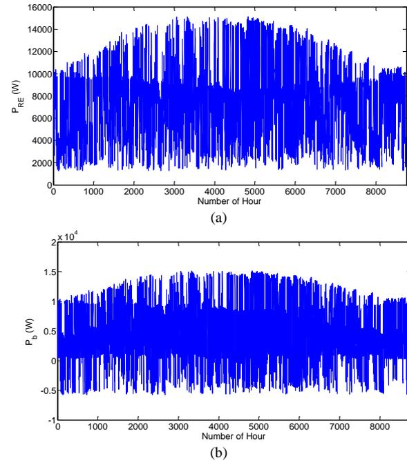
**Fig. 9. (a) Generated power by renewable resources ( $P_{RE}$ ), (b) Battery power input/output power during the year.**
