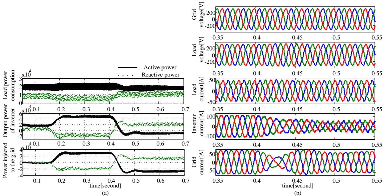
**Fig. 10. Inverter with LC-L filter. A simulation results of power reference step change. (a) From down: power injected to the grid, inverter power, load power. The active and reactive power at the load, inverter and grid. (b) From down: The waveforms of the grid current, inverter current, load current, load voltage and grid voltage.**
