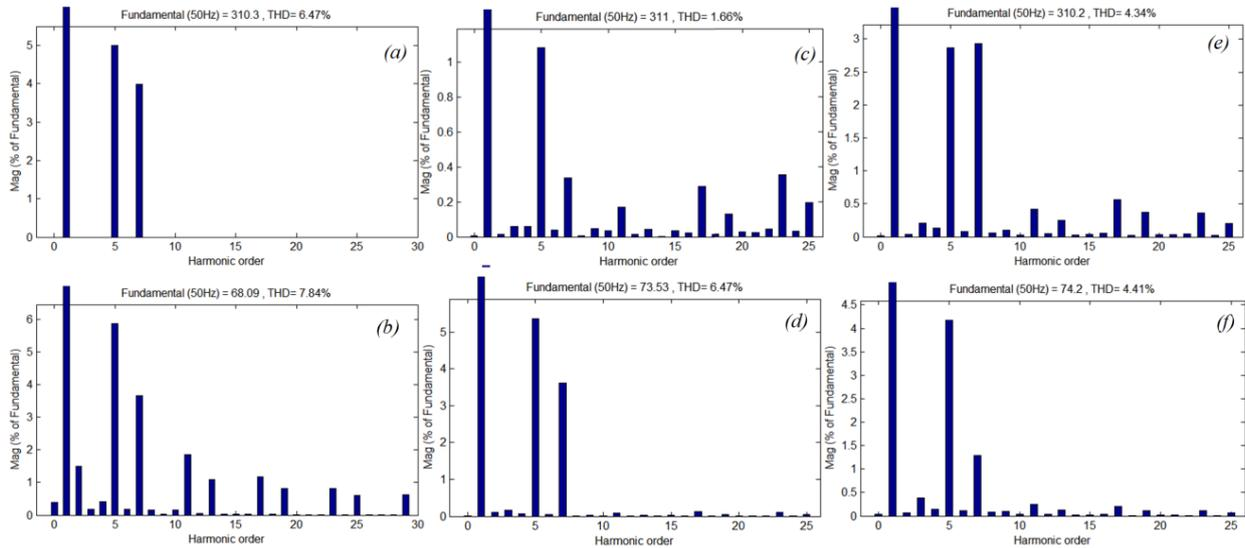
**Fig. 8. Fourier spectrum of the simulation results for the grid-connected mode:**
