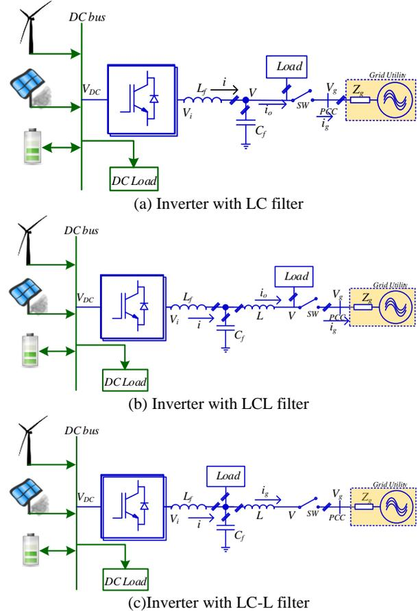
**Fig.1. Single line diagram of possible structures of Inverter.**
