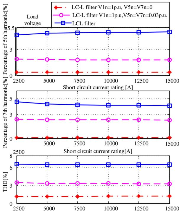
Fig. 11: Simulation results of load voltage for the grid-connected mode. From up: Percentage of fifth harmonic, Percentage of seventh harmonic and THD.
