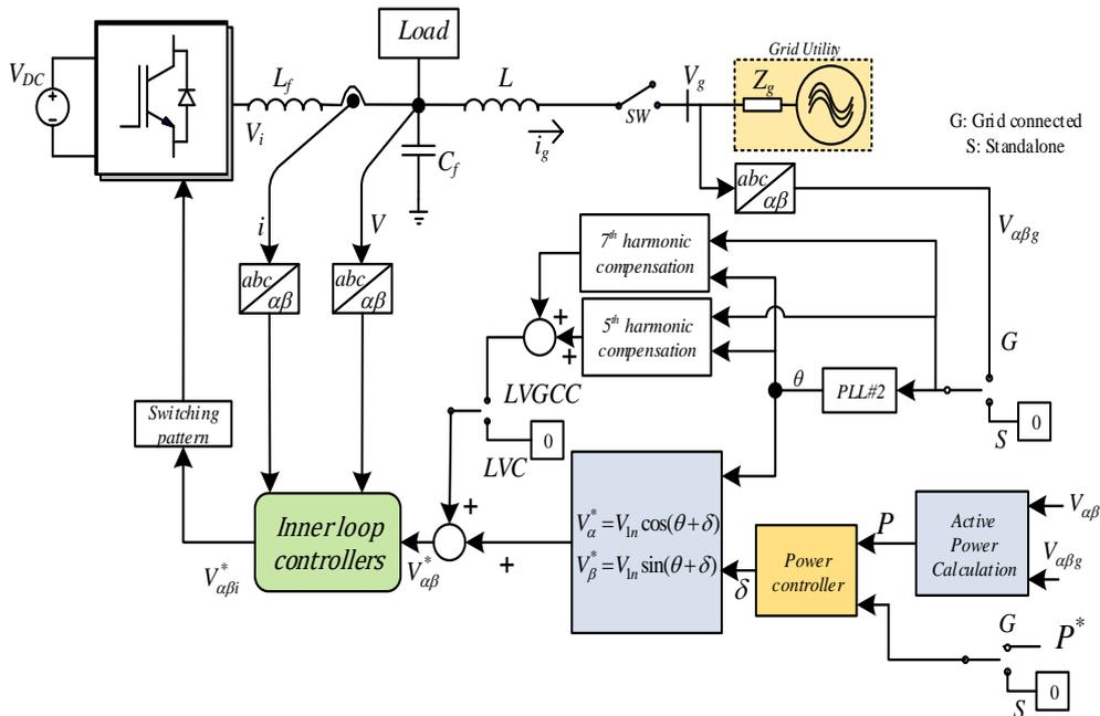
Fig. 3. Proposed inverter with LC-L filter: circuit diagram and implementation of the proposed control strategy.
