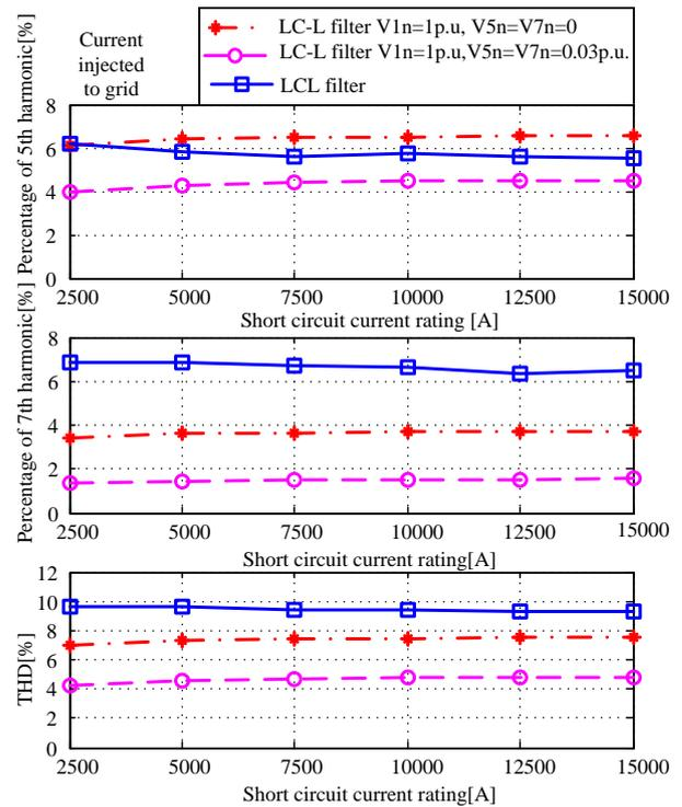
Fig. 12: Simulation results of current injected to grid for the grid-connected mode. From up: Percentage of fifth harmonic, Percentage of seventh harmonic and THD.
