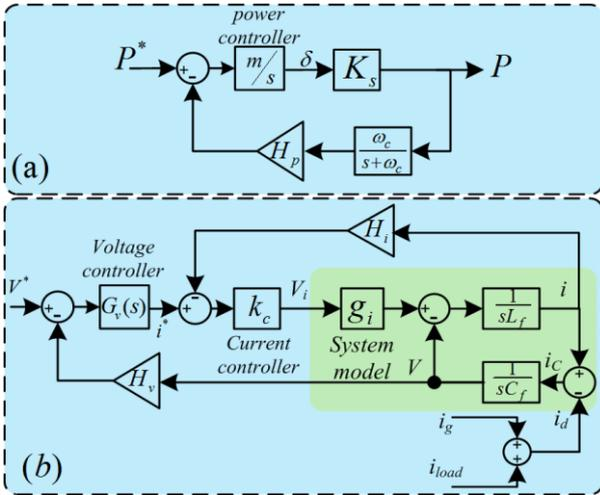
Fig. 4. (a) Power loop. (b) Inner loops for tracking of voltage reference in proposed inverter with LC-L filter in the stationary reference frame.
