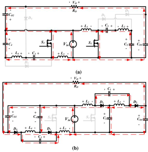
Fig. 4. Current flow path of operating modes during one switching period in CCM operation, (a) Mode 1, and (b) Mode 2.
