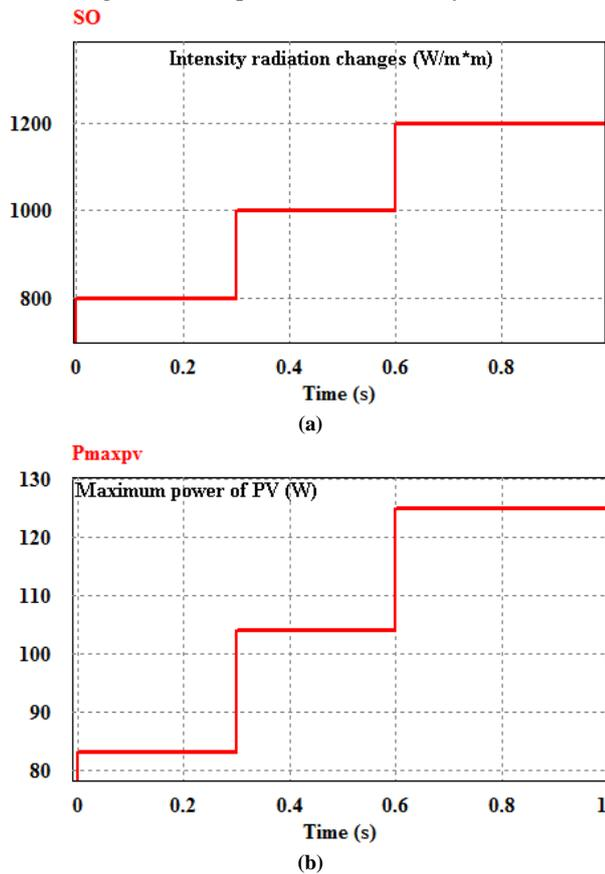
Fig. 11. Simulation results, (a) applied changes in intensity radiation, and (b) maximum PV power diagram for each three intensity radiations.
