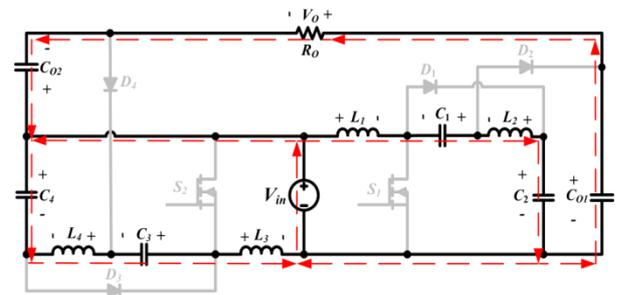
Fig. 6. Current flow path of proposed converter in third mode in DCM operation.
