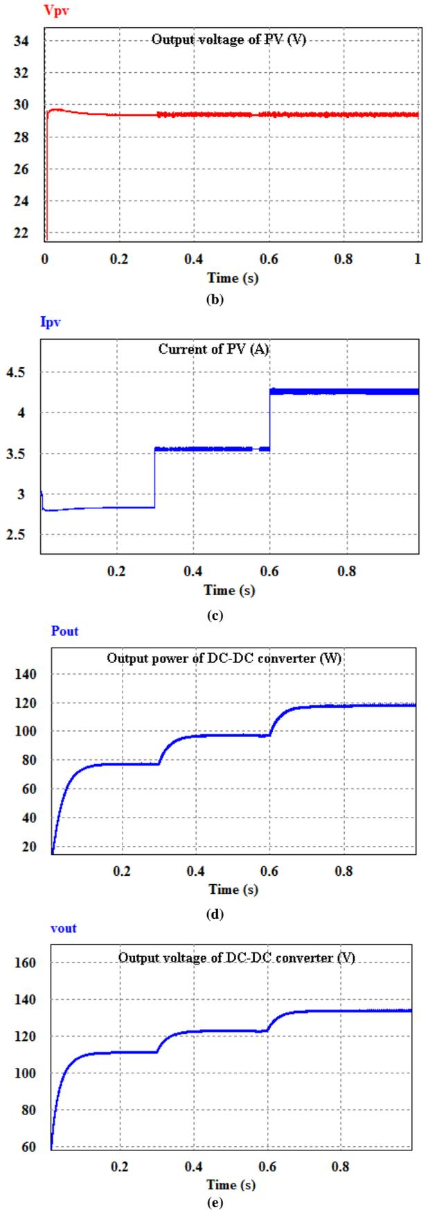
Fig. 12. Simulation results, (a) output power of PV, (b) output voltage of PV, (c) current of PV, (d) output power of DC-DC converter, and (e) output voltage of DC-DC converter.
