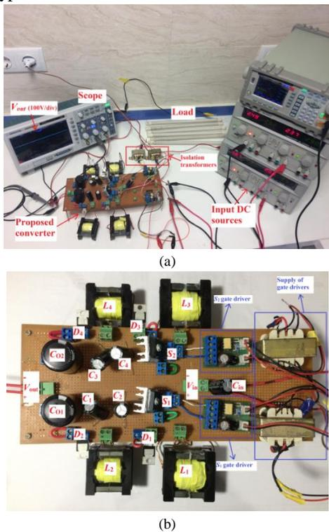
Fig. 13. Implemented prototype of proposed DC-DC converter, (a) overall system, and (b) power circuit.
