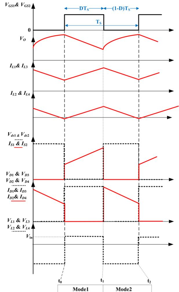
Fig. 3. Key waveforms of proposed converter operation in CCM.
