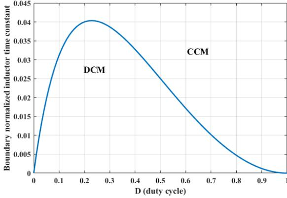
Fig. 7. Boundary normalized inductor time constant versus duty cycle.
