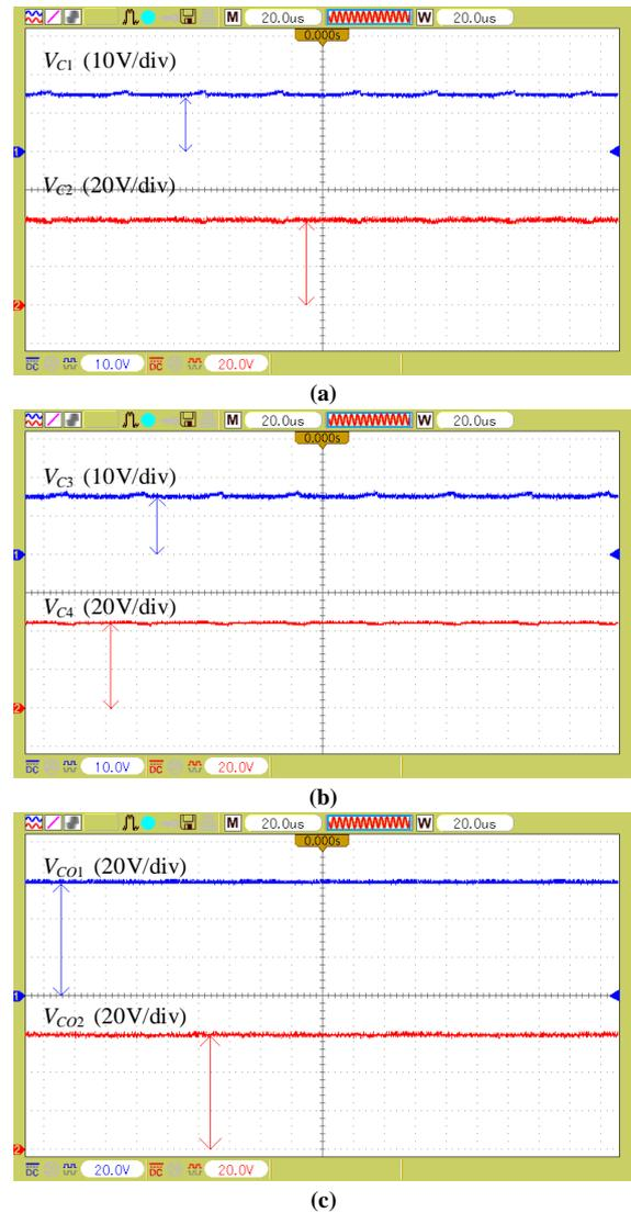
**Fig. 20.** Measured voltage waveforms of capacitors in DCM operation, (a)  $C_1$  and  $C_2$ , (b)  $C_3$  and  $C_4$ , and (c)  $C_{01}$  and  $C_{02}$
