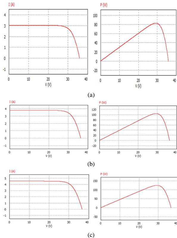
Fig. 10. I-V and P-V characteristic curves of the PV array, (a) 800 W/m<sup>2</sup>, (b) 1000 W/m<sup>2</sup>, and (c) 1200 W/m<sup>2</sup>.
