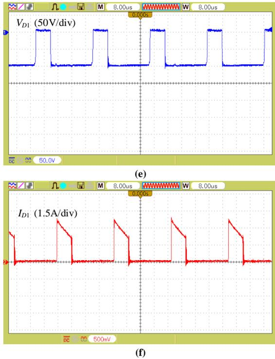
**Fig. 14.** Experimental measurement results of proposed DC-DC converter at CCM operation, (a) input and output voltages, (b) input current, (c) voltage of switch  $S_1$ , (d) current of switch  $S_1$ , (e) voltage of diode  $D_1$ , and (f) current of diode  $D_1$ .
