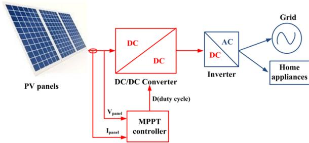
Fig. 1. General structure of a photovoltaic power system.
