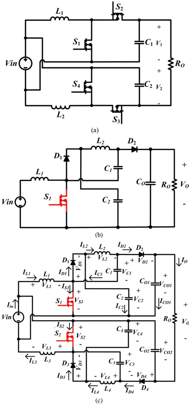
Fig. 2. (a) Base version of proposed interleaved double dual boost converter in [29], (b) Structure of modified step up KY converter, and (c) proposed interleaved DC-DC converter power circuit.
