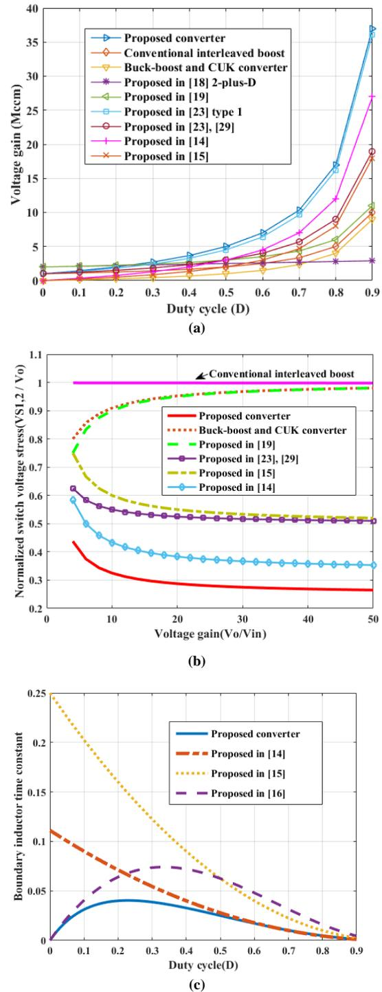
Fig. 8. Comparison results of proposed DC-DC converter with some similar step up topologies: (a) voltage gain of different topologies for various duty cycles, (b) normalized voltage stress of switches versus voltage conversion ratio in different topologies, and (c) curves of boundary inductor time constant.
