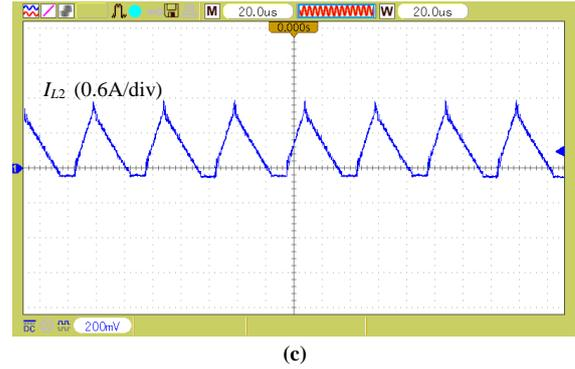
**Fig. 19.** Experimental measurement results in DCM operation: measured waveforms of (a) inductor  $L_1$  voltage, (b) inductor  $L_1$  current, and (c) inductor  $L_2$  current.
