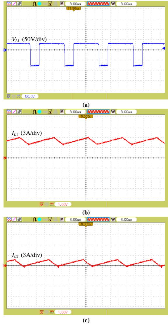
**Fig. 15.** Measured waveforms of (a) inductor  $L_1$  voltage, (b) inductor  $L_1$  current, and (c) inductor  $L_2$  current.
