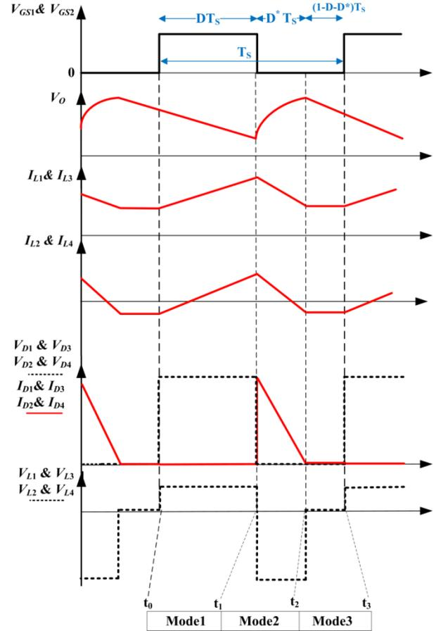
Fig. 5. Key waveforms of proposed converter operation in DCM.
