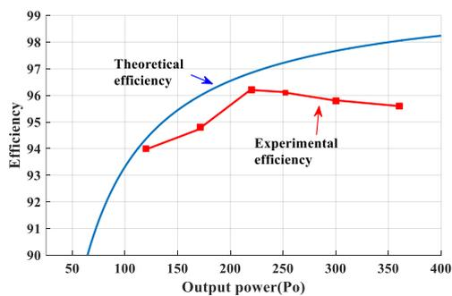
Fig. 17. Theoretical and experimental measured efficiency of proposed converter for  $R_{L1,3}=40\text{m}\Omega, R_{L2,4}=30\text{m}\Omega, r_{CO1,2}=10\text{m}\Omega, r_{C1,4}=10\text{m}\Omega, f_s=30\text{kHz}, C_s=603\text{pF}, V_{FD1,2,3,4}=1.2\text{V}, V_o=325\text{V}, P_o=220\text{W}$ .
