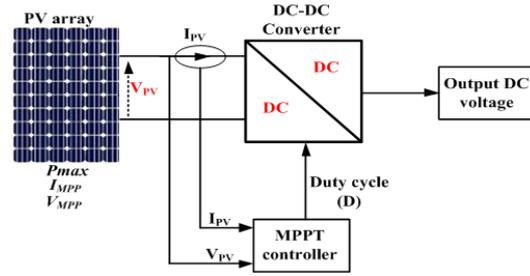
Fig. 9. General structure of simulated system in the PSIM.
