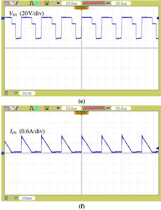
**Fig. 18.** Experimental measurement results of proposed DC-DC converter operation in DCM, (a) output voltage, (b) input current, (c) voltage of switch  $S_1$ , (d) current of switch  $S_1$ , (e) voltage of diode  $D_1$ , and (f) current of diode  $D_1$ .
