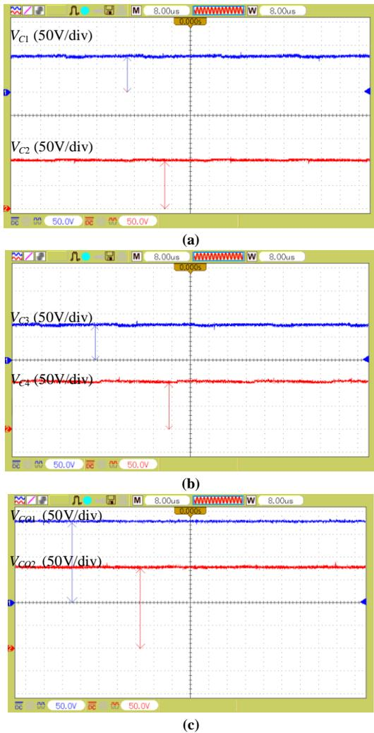
Fig. 16. Measured voltage waveforms of capacitors, (a)  $C_1$  and  $C_2$ , (b)  $C_3$  and  $C_4$ , and (c)  $C_{O1}$  and  $C_{O2}$ .
