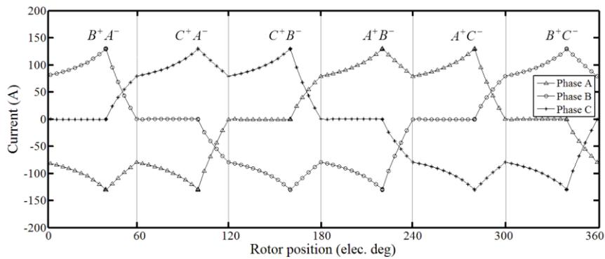
**Fig. 6.** Phase winding currents for 33-slot/34-pole BLDC motor
