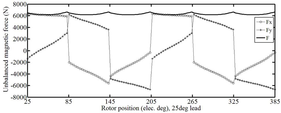
Fig. 16. X, y and resultant components of UMF in the 33-slot/34-pole BLDC motor in presence of 25 degrees of phase advance angle.
