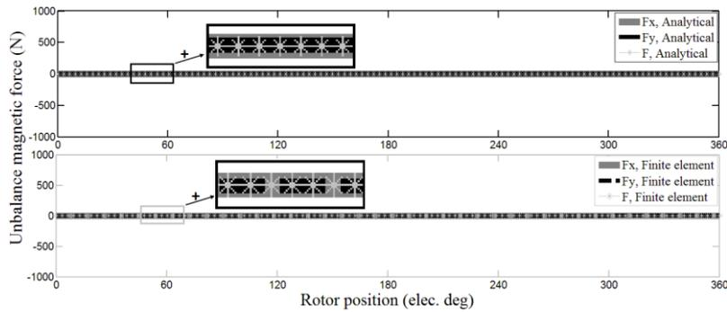
**Fig. 10.** UMF in the 36-slot/34-pole BLDC motor.
