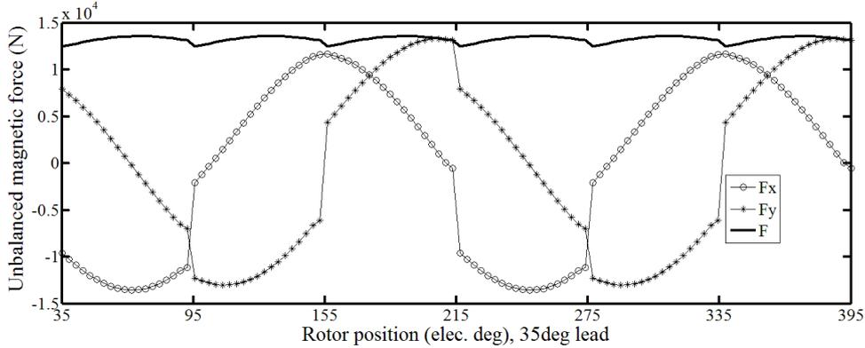
Fig. 18. X, y and resultant components of UMF in the 33-slot/34-pole BLDC motor in presence of 35 degrees of phase advance angle.
