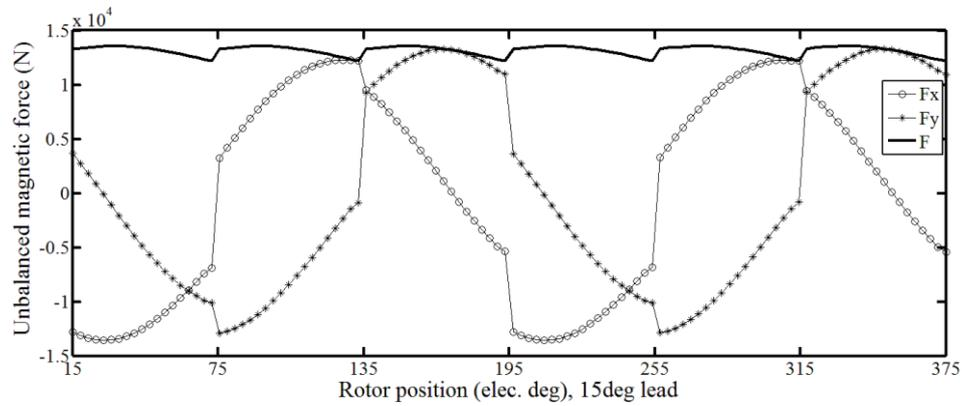
Fig. 14. X, y and resultant components of UMF in the 33-slot/34-pole BLDC motor in presence of 15 degrees of phase advance angle.
