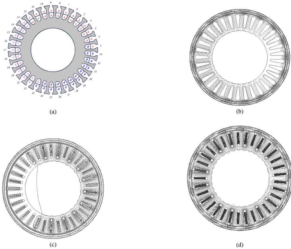
**Fig. 2.** Disposition of phase winding and display of flux lines in 33-slot/34-pole BLDC motor ( $i_a = +79.44 A$ ,  $i_b = -79.44 A$  and  $i_c = 0$ ). (a) Winding disposition. (b) Open circuit. (c) Armature reaction. (d) Resultant.
