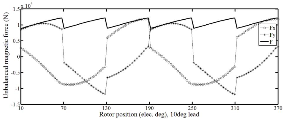
Fig. 13. X, y and resultant components of UMF in the 33-slot/34-pole BLDC motor in presence of 10 degrees of phase advance angle.
