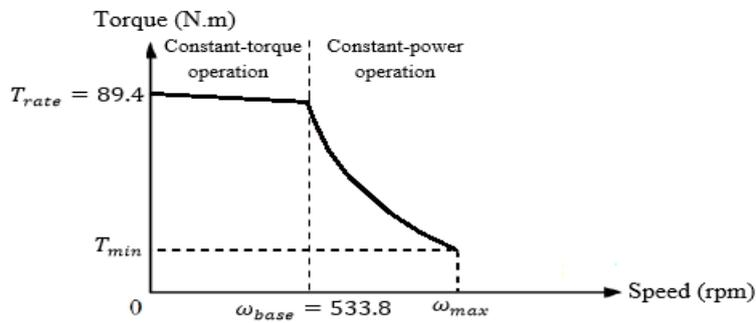
**Fig. 11.** Torque-speed curves.
