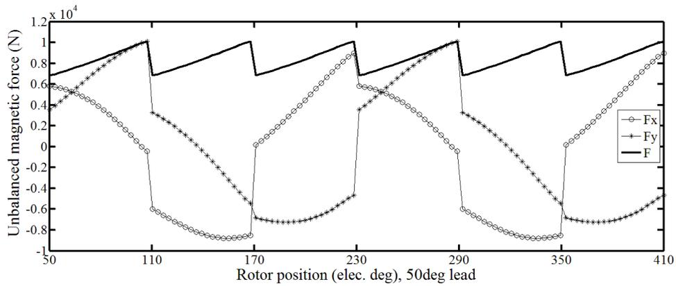
Fig. 21. X, y and resultant components of UMF in the 33-slot/34-pole BLDC motor in presence of 50 degrees of phase advance angle.
