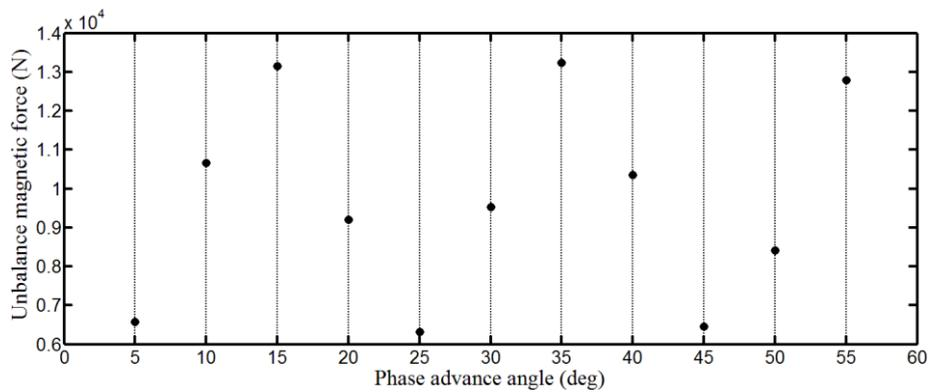
Fig. 23. Average amount of UMFs for each phase advance angle value in the 33-slot/34-pole BLDC machine.
