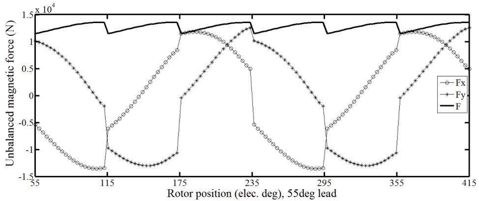
Fig. 22. X, y and resultant components of UMF in the 33-slot/34-pole BLDC motor in presence of 55 degrees of phase advance angle.
