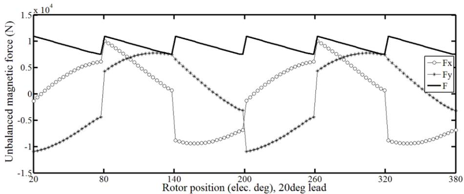
Fig. 15. X, y and resultant components of UMF in the 33-slot/34-pole BLDC motor in presence of 20 degrees of phase advance angle.
