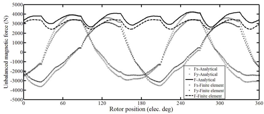
**Fig. 5.** UMF in the 33-slot/34-pole BLDC motor
