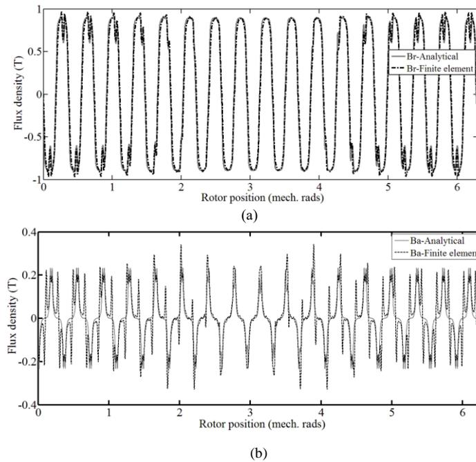
**Fig. 3.** Permanent magnet field distribution on the middle of the air-gap for 33-slot/34-pole BLDC motor. (a) Radial (b). Tangential.
