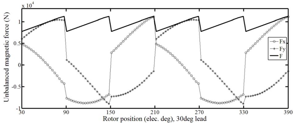
Fig. 17. X, y and resultant components of UMF in the 33-slot/34-pole BLDC motor in presence of 30 degrees of phase advance angle.
