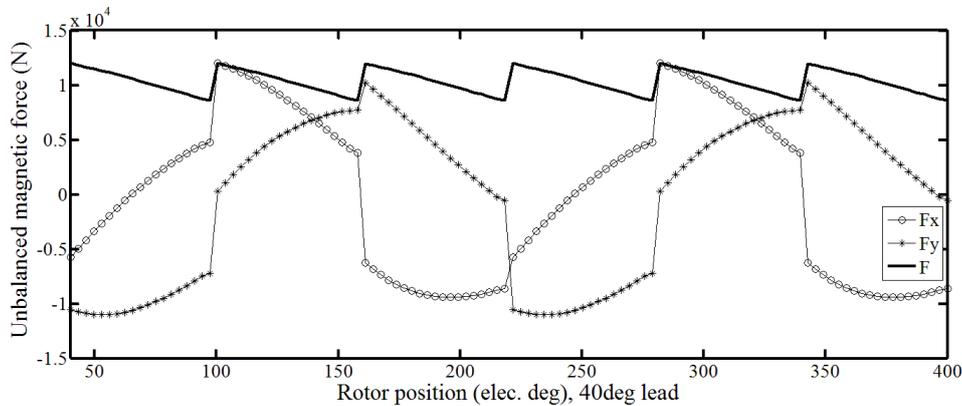
Fig. 19. X, y and resultant components of UMF in the 33-slot/34-pole BLDC motor in presence of 40 degrees of phase advance angle.
