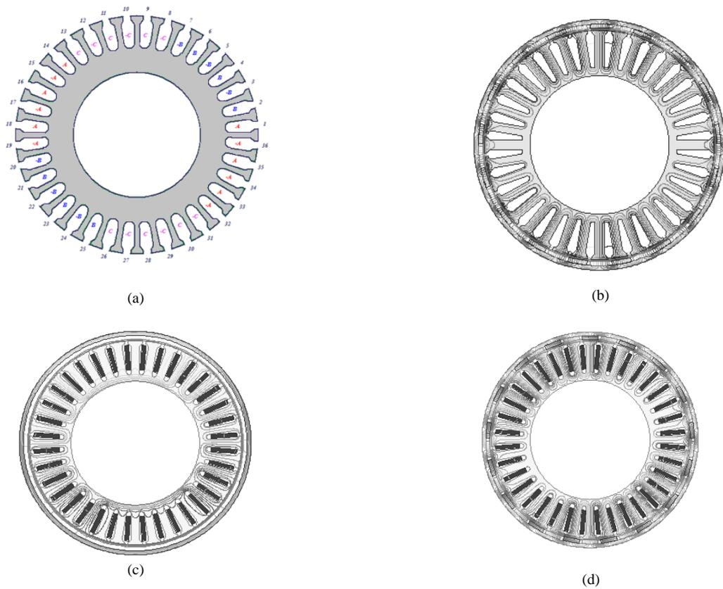
**Fig. 7.** Disposition of phase winding and display of flux lines in 36-slot/34-pole BLDC motor ( $i_a = +79.44$ ,  $i_b = -79.44$  and  $i_c = 0$ ). (a) Winding disposition. (b) Open circuit. (c) Armature reaction. (d) Resultant.
