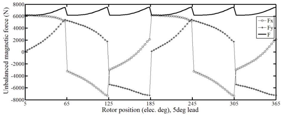
Fig. 12. X, y and resultant components of UMF in the 33-slot/34-pole BLDC motor in presence of 5 degrees of phase advance angle.
