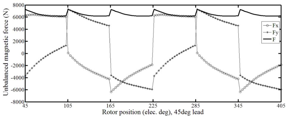
Fig. 20. X, y and resultant components of UMF in the 33-slot/34-pole BLDC motor in presence of 45 degrees of phase advance angle.
