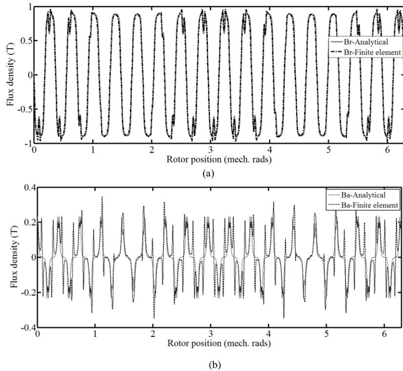
**Fig. 8.** Permanent magnet field distribution on the middle of the air-gap for 36-slot/34-pole BLDC motor. (a) Radial, (b) Tangential.
