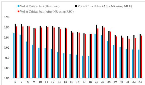
Fig. 5. Comparison of voltage magnitudes at critical buses before and after NR of 33 bus RDS.
