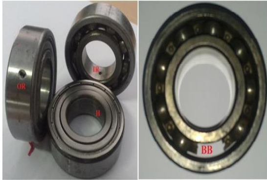
Fig. 4. Healthy bearing (H), Outer race fault (OR), Inner race fault (IR), Ball broken fault bearing (BB).
