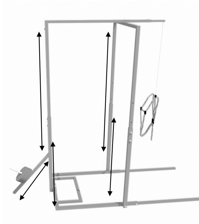
Figure 3. Placing the columns sliding inside each other and fixing them with bolts and nuts
