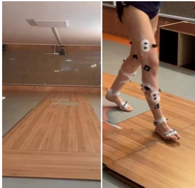
Figure 1. The present discourse presents an extended perspective of the Laboratory of Biomechanics with a focus on the walkway. The walkway is equipped with a sophisticated motion-capture system that includes state-of-the-art cameras and force plates.
