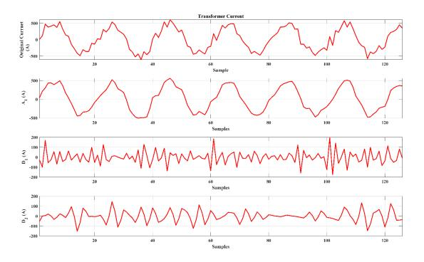
Fig. 2. Applying the wavelet transform on the input current of the transformer
