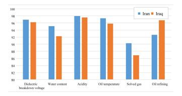
Fig. 8. The effect of oil quality parameters on the accuracy of life estimation
