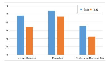
Fig. 7. The effect of power quality parameters on the accuracy of life estimation
