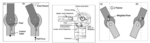
Figure 18. Locking System Design of Ratchet/Pawl In Spring and Weight (32)
