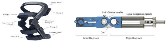
Figure 5. (A) Spring Loaded Knee Brace; (B) Hinge and Energy Storage Mechanism (14, 15)
