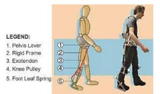
Figure 1. Schematic Of XPED2 Conceptual Design, Introduction Components & Skeleton Worn by User (7)
