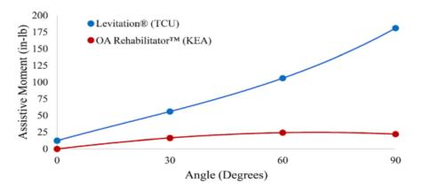
Figure 7. Comparison Of Guardian and Levitation Auxiliary Torque Knee Joint (13)
