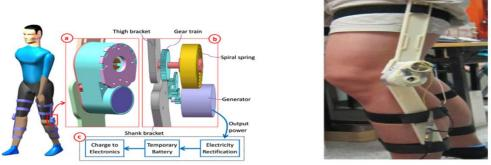
Figure 4. Image and CAD Model Of Harvester Energy System Made Via Rapid Prototyping Method (12)
