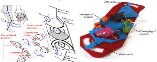
Figure 12. Isometric Images of Left Prototype Mechanism and Right Rapid Prototype (23)
