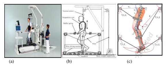
Figure 16. (a): Hocoma AG's Lokomat; (b) and (c): Alamdari Proposed Cable-Based Robot Design (27)
