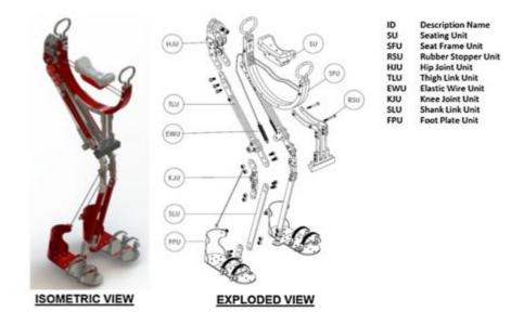
Figure 3. Isometric View and Explosion Map Of WAE Passive Skeleton CAD Model (11)
