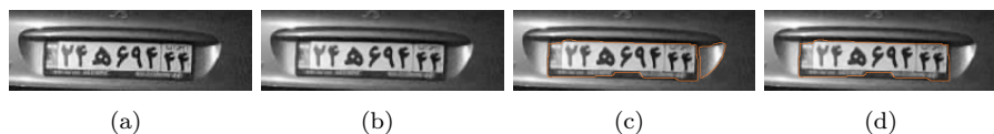
Figure 1. (a) A gray scaled license plate (b) Smoothed version of (a) (c) All closed curves around minimal surfaces (d) Closed curve with maximum area
