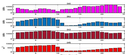
**Fig. 14. SoC of storages at each hour in Case study 4 (a) TESS , (b) CAES , (c) ISC , (d) water tank**
