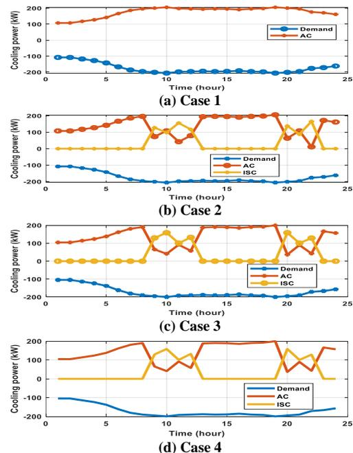
Fig. 12. Optimal dispatch outcomes of cooling flow at cooling hub under the four cases considered in the study
