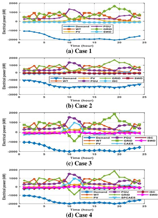
Fig. 10. Optimal dispatch outcomes of the power flow at electrical hubs under the four cases considered in the study
