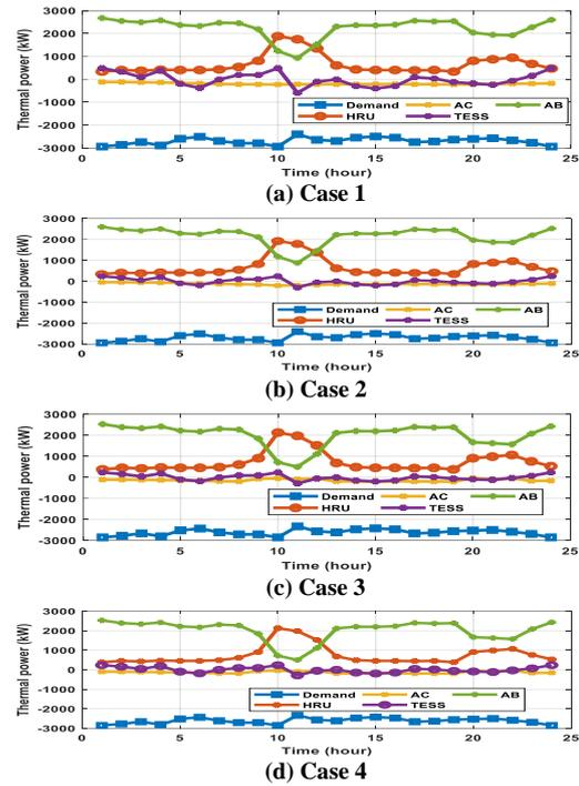
Fig. 11. Optimal dispatch outcomes of thermal flow at thermal hub under the four cases considered in the study
