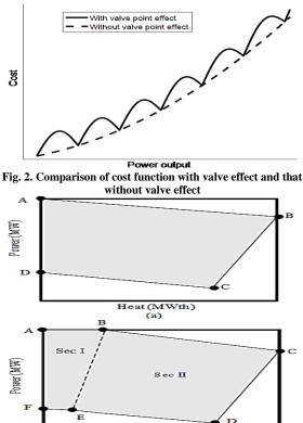
Heat(MWth) (b) Fig. 3. Heat-power feasible operation region of a CHP unit
