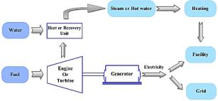
Fig. 1. Common configuration of a CHP
